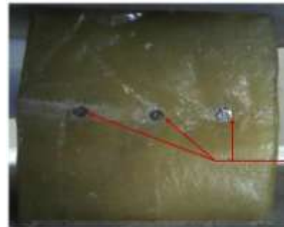
Figure 5.2: Debonding of fibers at 0 degree orientation
