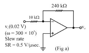
Determine the maximum frequency of operation.
